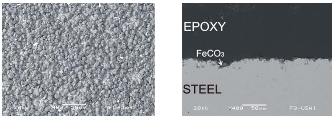
Figure 12 . Baseline experiment without in pure CO 2 solution after 240h of exposure (pCO 2 =0.56 bar, pH 6.6, T=80°C). a) FeCO 3 scale morphology, frontal view and b) FeCO 3 scale thickness, cross section.
