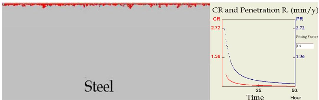
Figure 14. Surface morphology and the trend of the corresponding uniform corrosion rate (lower curve denoted CR) and localized penetration rate (upper curve denoted PR) as predicted by 2-D model at 50 ppm  $\text{Fe}^{2+}$ , 0.54bar  $\text{pCO}_2$ , 80 °C, pH 6.6, and 1m/s.
