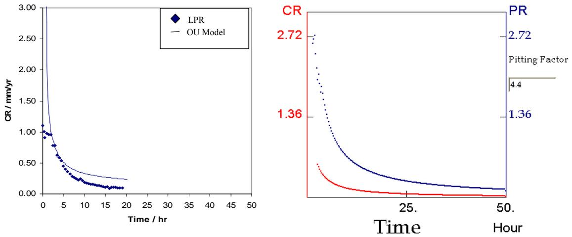
Figure 7. Comparison of corrosion rate obtained from 1-D prediction model<sup>(12,13,14)</sup>, LPR experimental data<sup>(19)</sup> (shown on the graph on the left) and the present 2-D prediction (shown on the graph on the right) including prediction of uniform corrosion (lower curve denoted CR), localized pit penetration rate (upper curve denoted PR) and pitting factor ( $f=4.4$ ). Conditions: pH 6.6, 80°C, 0.52bar  $P_{CO_2}$ , 50ppm  $Fe^{2+}$ , and stagnant.
