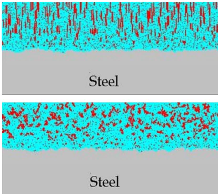
Figure 2. Comparison of the film morphology before (top) and after (bottom) using a random film formation algorithm at pH 6.6, 80°C, 5ppm  $\text{Fe}^{2+}$  and 0.52bar  $\text{pCO}_2$ .
