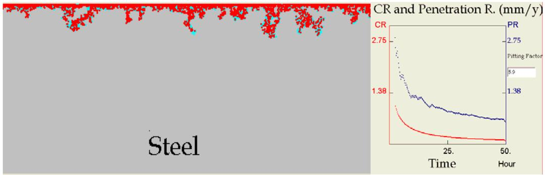
Figure 12. Surface morphology and the trend of the corresponding uniform corrosion rate (lower curve denoted CR) and localized penetration rate (upper curve denoted PR) as predicted by 2-D model at 28 ppm  $\text{Fe}^{2+}$ , 0.54bar  $\text{pCO}_2$ , 80 °C, pH 6.6, and 1m/s.
