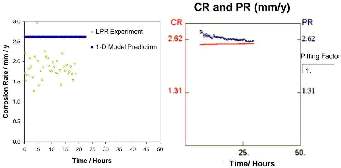
Figure 5. Comparison of corrosion rate obtained from 1-D prediction model<sup>(12,13,14)</sup>, LPR experimental data<sup>(19)</sup> (shown on the graph on the left) and the present 2-D prediction (shown on the graph on the right) including prediction of uniform corrosion (lower line denoted CR), localized pit penetration rate (upper curve denoted PR) and pitting factor ( $f=1$ ). Conditions: pH 6.0, 80°C, 0.52bar  $P_{CO_2}$ , 50ppm  $Fe^{2+}$ , and stagnant.
