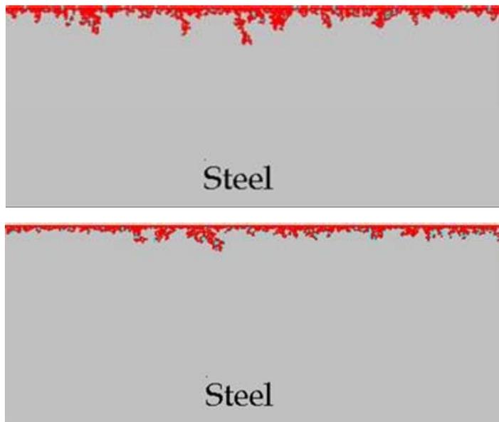
Figure 4. Comparison of the film morphology before (top) and after (bottom) using a random film formation algorithm at pH 6.5, 80°C, 50ppm  $\text{Fe}^{2+}$  and 0.52bar  $p_{\text{CO}_2}$ .
