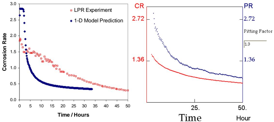
Figure 6. Comparison of corrosion rate obtained from 1-D prediction model<sup>(12,13,14)</sup>, LPR experimental data<sup>(19)</sup> (shown on the graph on the left) and the present 2-D prediction (shown on the graph on the right) including prediction of uniform corrosion (lower curve denoted CR), localized pit penetration rate (upper curve denoted PR) and pitting factor ( $f=1.3$ ). Conditions: pH 6.3, 80°C, 0.52bar  $P_{CO_2}$ , 50ppm  $Fe^{2+}$ , and stagnant.
