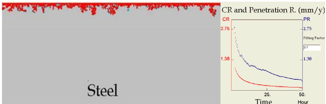
Figure 13. Surface morphology and the trend of the corresponding uniform corrosion rate (lower curve denoted CR) and localized penetration rate (upper curve denoted PR) as predicted by 2-D model at 30 ppm  $\text{Fe}^{2+}$ , 0.54bar  $\text{pCO}_2$ , 80 °C, pH 6.6, and 1m/s.
