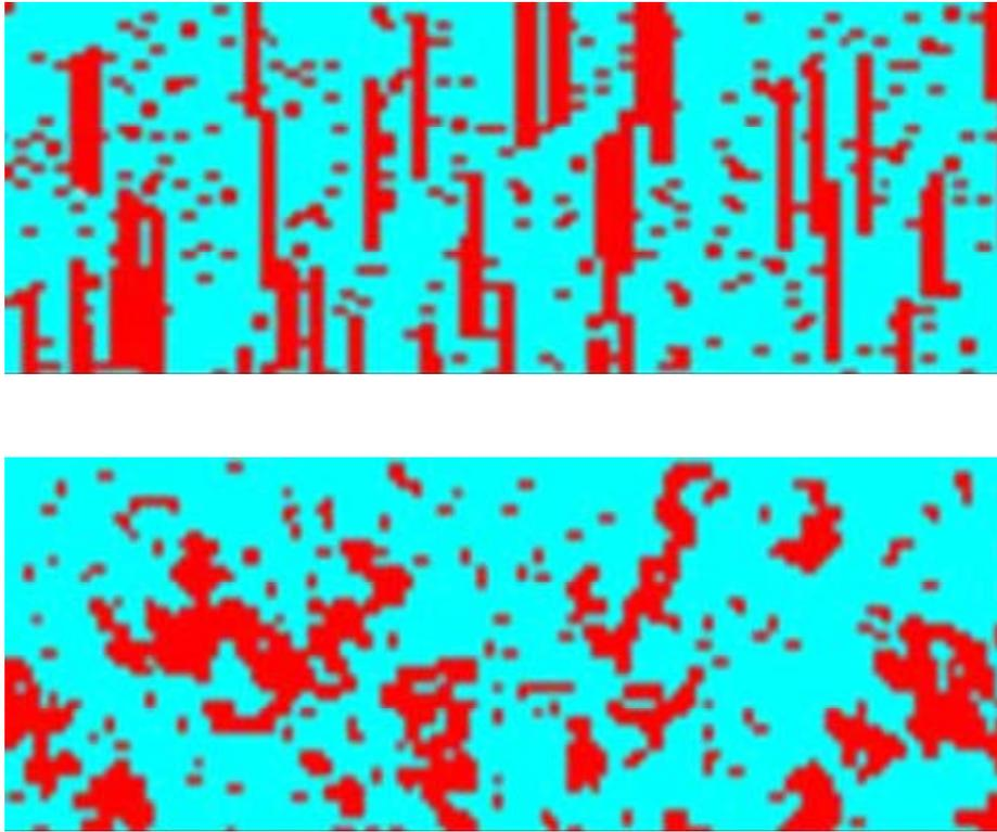
Figure 3. Comparison of the film morphology at higher magnification before (top) and after (bottom) using a random film formation algorithm at pH 6.6, 80°C, 5ppm  $\text{Fe}^{2+}$  and 0.52bar  $p_{\text{CO}_2}$ .
