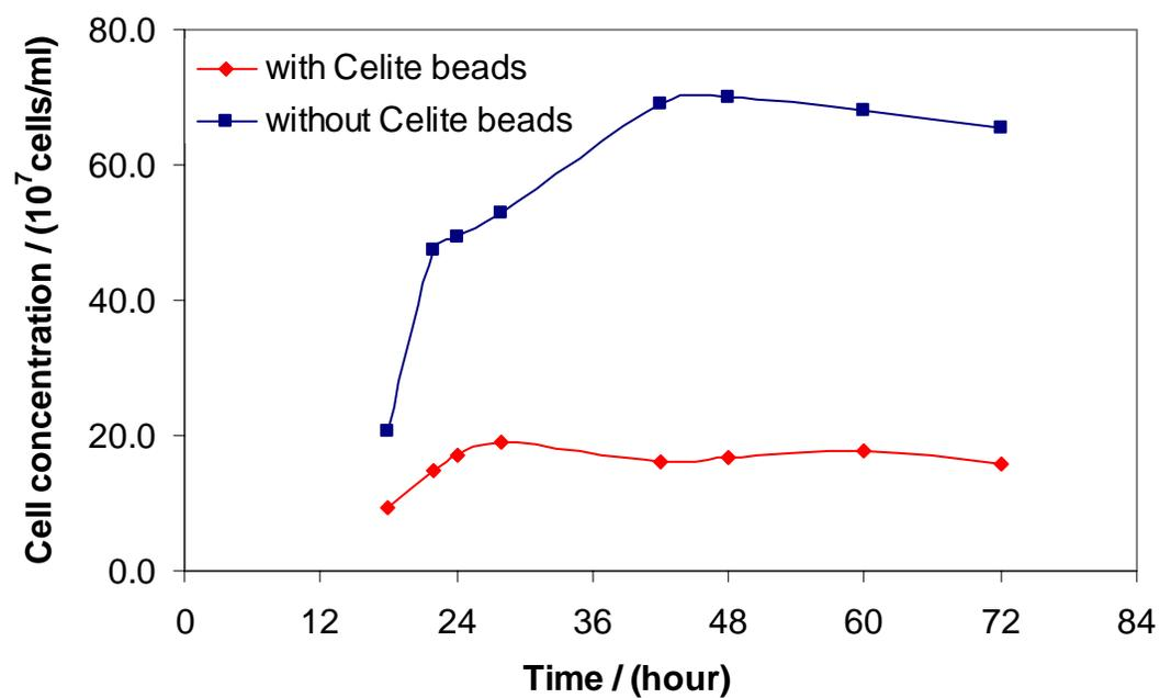
FIGURE 11 - SRB planktonic cell counts with and without Celite beads in a medium with a 25 ppm initial Fe<sup>2+</sup> concentration in a 2-L glass cell.
