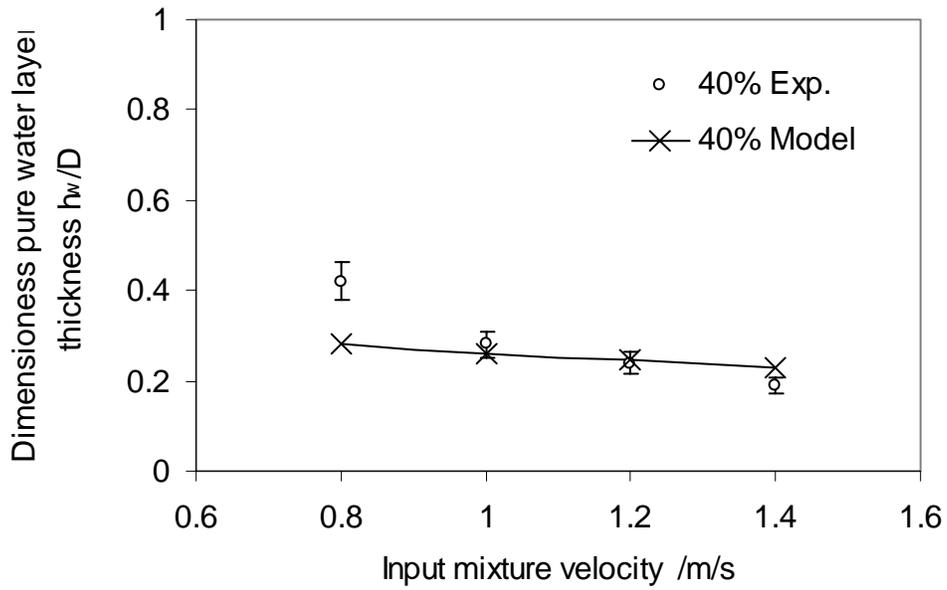
FIGURE 5. Comparison between the predicted results by the model and experimental data of pure water layer thickness (Shi et al.<sup>30</sup>) at input water cut of 40%.
