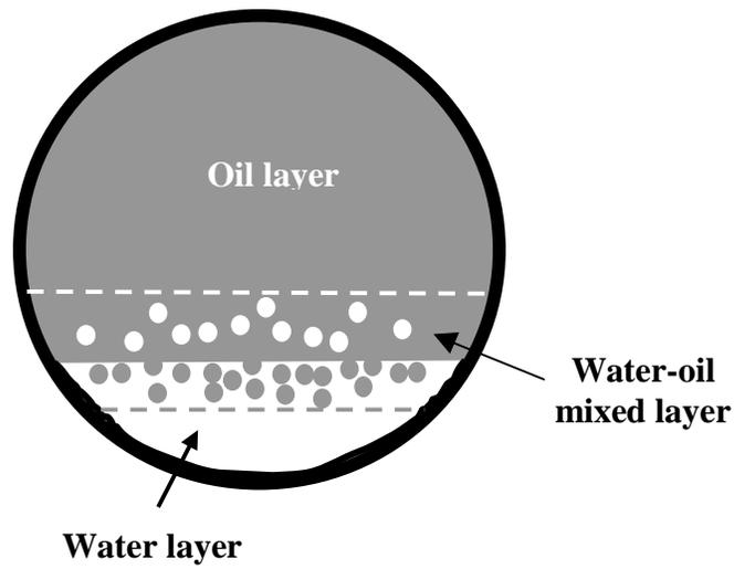
FIGURE 2. Cross-section for a three-layer flow structure with a planar interface
