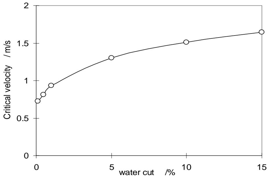
FIGURE 6. Effect of water cut on critical velocity at  $\rho_o=820 \text{ kg/m}^3$ ,  $\mu_o=2 \text{ cP}$
