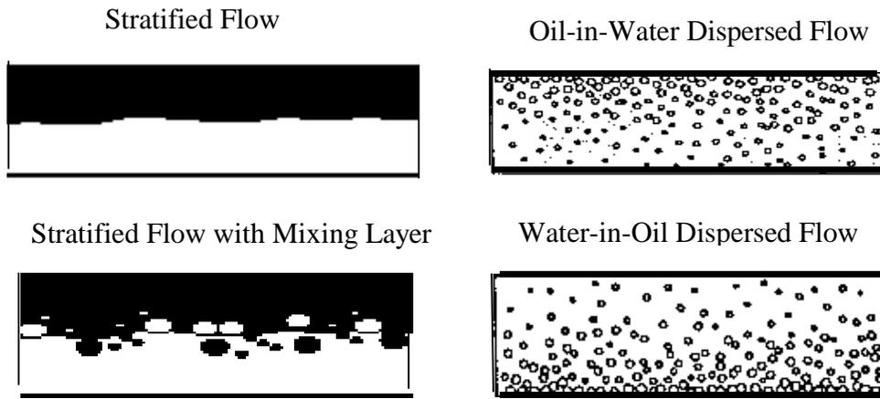
FIGURE 1. Flow patterns in oil-water horizontal flows
