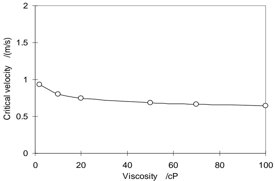
FIGURE 10. Effect of viscosity on critical velocity at  $D=0.1$  m,  $\sigma=0.029$  N/m, water cut=1% and  $\rho_o=820$  kg/m<sup>3</sup>
