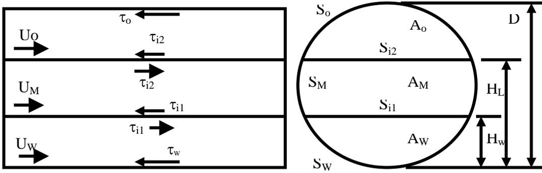
FIGURE 3. Schematic representation of the three-layer segregated oil-water flow
