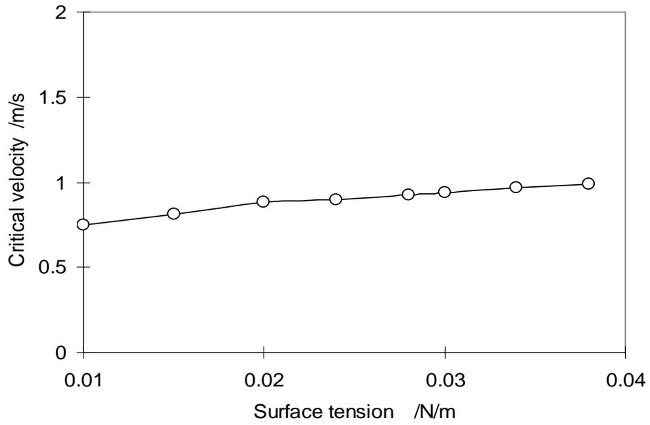
FIGURE 9. Effect of surface tension on critical velocity at  $D=0.1$  m,  $\mu_o=2$  cP, water cut=1% and  $\rho_o=820$  kg/m<sup>3</sup>
