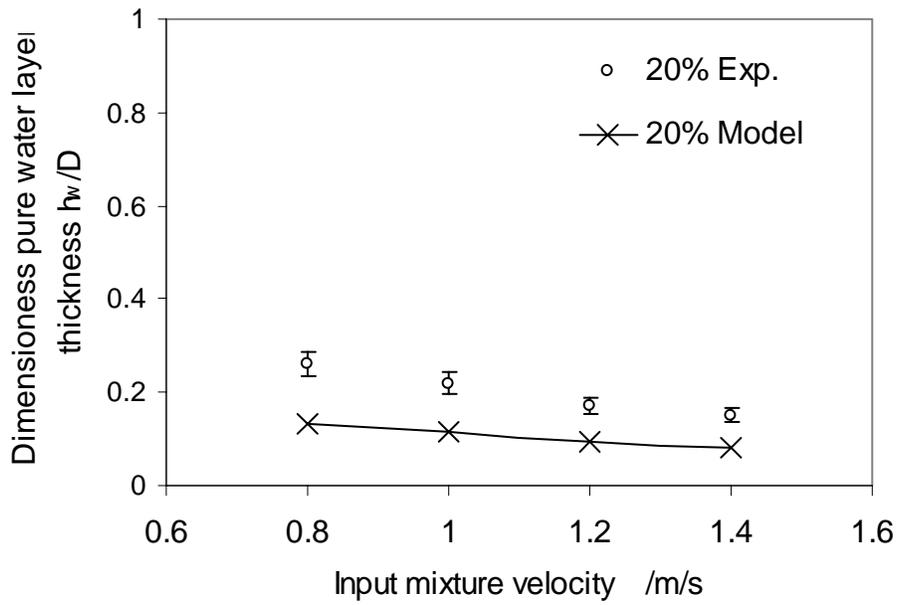
FIGURE 4. Comparison between the predicted results by the model and experimental data of pure water layer thickness (Shi et al.<sup>30</sup>) at input water cut of 20%.
